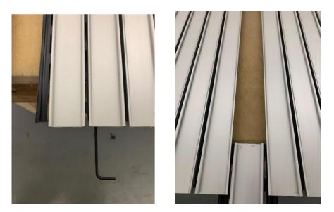
5. Once the sections of mat are lying next to each other, slide the removed rail back into place joining it with the hinge-receiving rail on the bottom of section "A" and the top of section "B."
